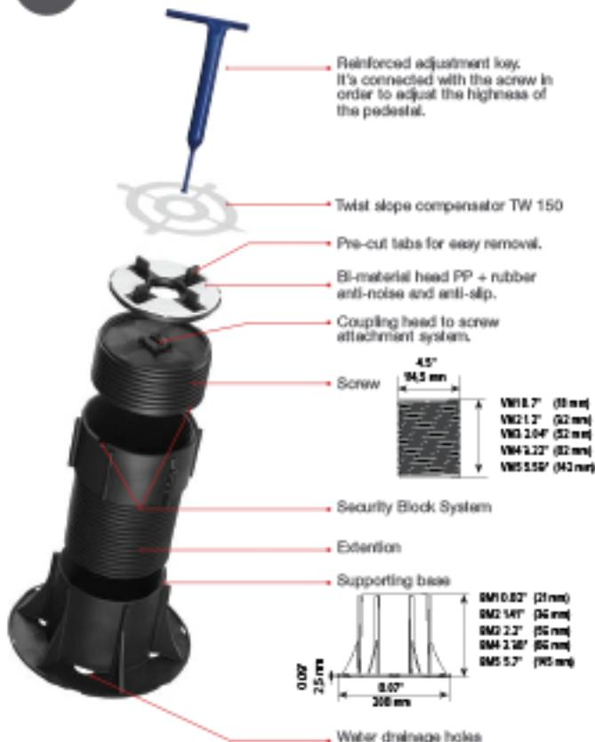
It boasts a wide range of features that make it perfect for any type of raised flooring applications, including noise-reducing rubber ends, a special adjustment wrench, variable heights and a pre-cut base for wall corner cuts.
